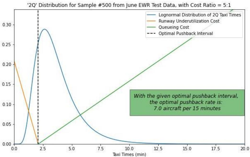
Figure 8. Sample Optimization Output with 5:1 Augmented Cost Ratio
