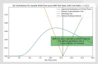
Under the same cost function ratio, the optimal pushback interval <a href="increases">increases</a> as the prediction of the 2Q taxi time—the scale of the lognormal distribution—increases.
