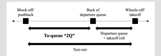
The departure taxi-out can be segmented into the queuing process and the unimpeded "2Q" time from gate pushback to entering the back of the departure queue
